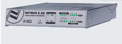
Interface and 16 channel audio level detector. It works as a mutichannel level detector for camera selection in Visual Radio systems. It reads the audio levels at its 4 analog, 4 digital and 8 Dante inputs and sends the reading to the AEQ VisualRplus Visual Radio system through the IP network. Dimensions: 1U x ½ 19", (207x41mm).
