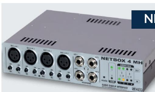
Provides 4 micro / line inputs, 4 line outputs and 4 stereo headphone outputs. Includes 4 GPI and 4 GPO, as well as additional GPIOs for signaling boxes such as Studiobox. It can be powered using PoE.
