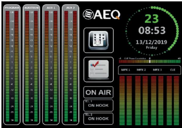
The most important vu-meters are located at the left and shown in maximum resolution. They have fixed names: PROGRAM, AUDITION, AUX 1 and AUX 2.
